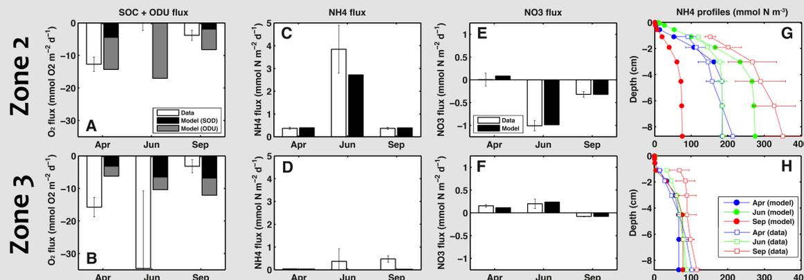
Figure 2. Comparison of observed and simulated SOC (A-B), sediment-water fluxes of NH<sub>4</sub> (C-D) and NO<sub>3</sub> (E-F), and sediment NH<sub>4</sub> concentrations (G-H) at Zone 2 (upper panels) and Zone 3 (lower panels) stations in April, June and September 2006. Error bars indicate the standard deviation of the observations.
