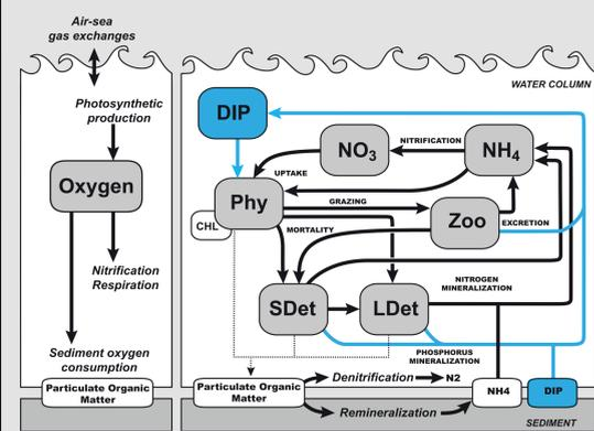
Figure 1. Schematic of the ecosystem model. Black arrows indicate the original nitrogen cycle model of Fennel et al. (2011) and blue arrows the added phosphorus processes (Laurent et al. 2012). Sedimenting particulate organic matter (dashed arrows) is instantly remineralized into ammonia and phosphate at the sediment-water interface. Part of the nitrogen is lost into nitrogen gas (N<sub>2</sub>) through denitrification. Oxygen sources and sinks are represented on the left-hand side panel.
